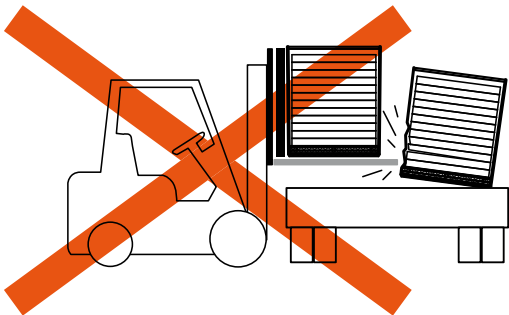
Fig.6 Too long forks may damage the second row of packages.
