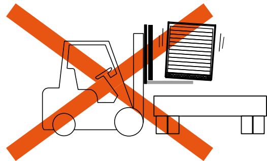
Fig.5 Too short forks may damage a package.
